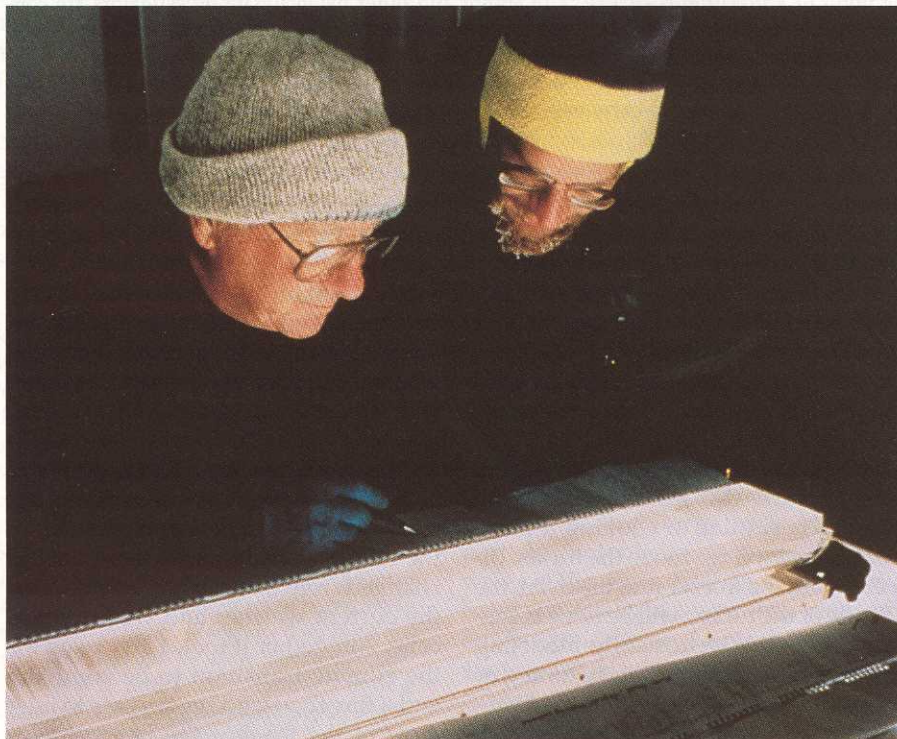
Figure 3. Richard Alley of Pennsylvania State University and Mark Meier of the University of Colorado count annual layers (light and dark bands about a centimeter apart) in an ice core. (Photograph courtesy of Ken Abbott/National Ice Core Laboratory.)
