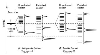
**Figure 6.** Exciton band structures and IR spectra of the antiparallel and parallel β-sheets in zero order, unperturbed and perturbed by  $^{13}$ C-substitution. The nearest-neighbor coupling along the strand is  $V_{ns,ns+1}$ .
