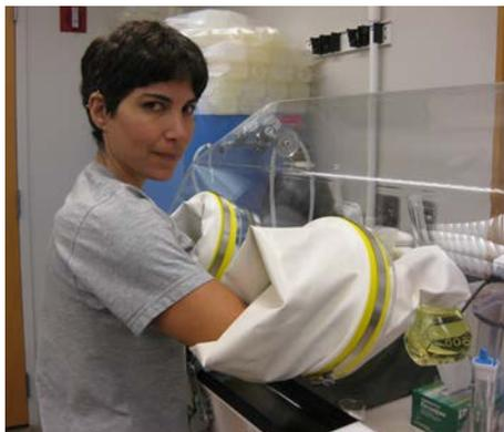
*Working with anoxic thiotungstate solution in glove box.*
