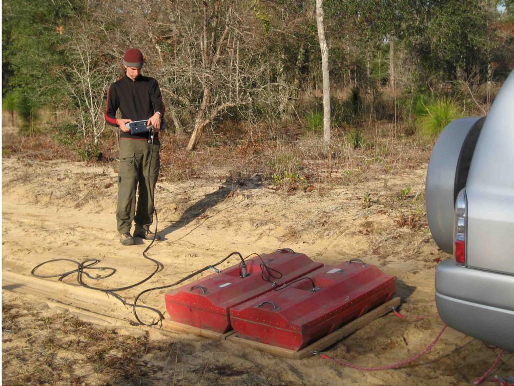
Figure S4: Configuration for the ground-penetrating radar survey. A 100 MHz bistatic radar antenna manufactured by Geophysical Survey Systems, Inc., was towed behind an automobile with an operator trailing the antenna and controlling the instrument with portable laptop.
