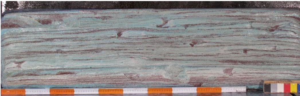
Figure 3. Physical stratigraphy of the highly cohesive delta at the proximal transect. Ruler at the bottom of the image has white and orange sections that are 10 cm long for scale. The color card in the bottom of the image provides a reference for color. Coarse sediment is colored red. The blue tint in the light sediment is from the dye used to color the input water.
