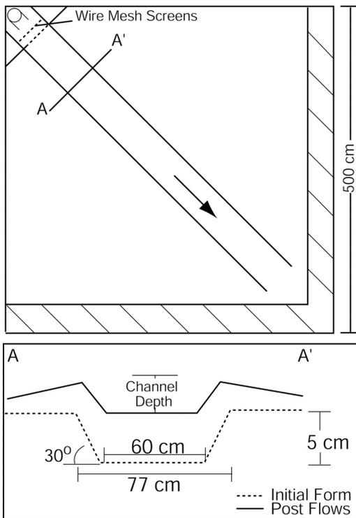
Figure 1. Setup for the straight channel experiment. (top) Plan view of straight channel configuration. Currents enter in top left corner of tank and pass through an excess-momentum diffuser before entering the channel. The moat running along far sidewalls of the tank is marked by a hatched pattern. Piping in the moat removes current from the tank, inhibiting reflections. (bottom) Initial form and an approximate final geometry of a channel cross-section.
