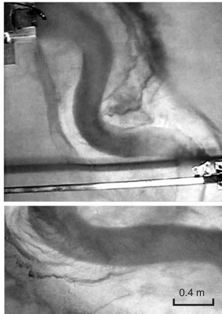
Figure 4.3. Turbidity current spilling onto the overbank surface along the outer banks of bend 1 (upper photo) and bend 2 (lower photo). Waves developed at the interface between the current and the ambient fluid are visible in the photograph from each bend. Overbank flow is visible from dye injected into the body at the beginning of the channel. Flow is from the upper left to lower right in both pictures.
