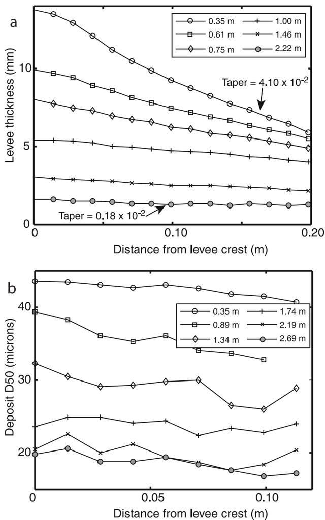
**Figure 11.** Cross-sectional profiles of the depositional levee at six different locations down the channel. (a) Levee thickness and taper decrease with increasing distance from the channel entrance. (b) D50 of levee deposit decrease with distance from channel entrance, but rate of D50 decrease with distance from levee crest changes negligibly with distance from channel entrance.
