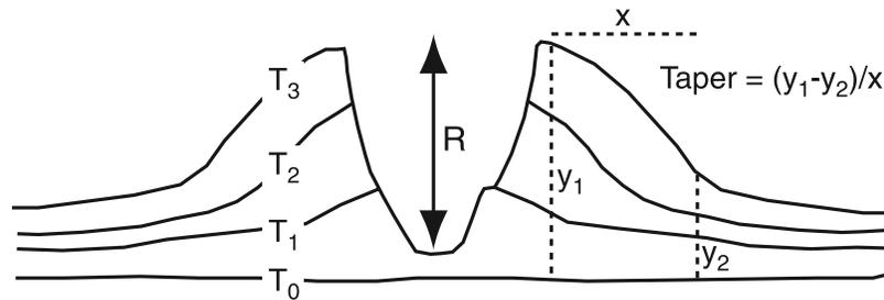
**Figure 1.** Definition sketch for the geometry of a levee.
