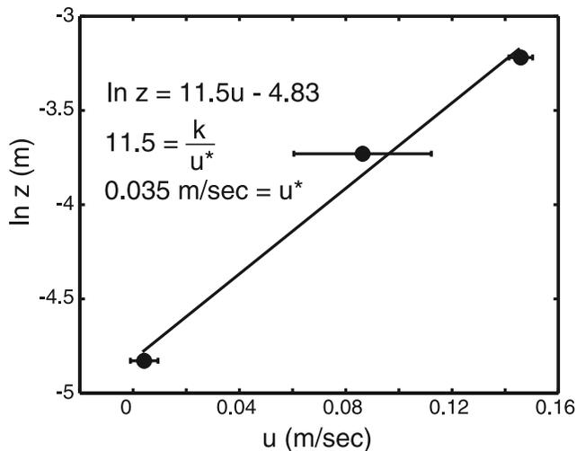
**Figure 10.** Estimation of model  $u^*$  obtained with best fit slope of  $\ln z$  versus current velocity plot. Velocity measurements were obtained below the velocity maximum of each sample profile. Horizontal error bars are  $\pm 1$  standard deviation calculated using all values for current velocity collected in each sampling volume;  $u^*$  value of the experimental flow events presented equals 0.035 m/s.
