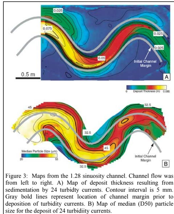
Figure 3: Maps from the 1.28 sinuosity channel. Channel flow was from left to right. A) Map of deposit thickness resulting from sedimentation by 24 turbidity currents. Contour interval is 5 mm. Gray bold lines represent location of channel margin prior to deposition of turbidity currents. B) Map of median (D50) particle size for the deposit of 24 turbidity currents.
