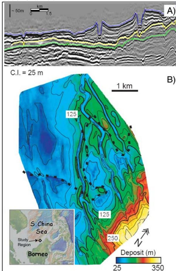
Figure 1: A) Characteristic strike-oriented seismic line for study region showing portion of the regional stratigraphy from the seafloor (blue line) to regional (Yellow) horizon. B) Deposit thickness measured between seafloor and regionally (Yellow) mapped subsurface horizon. Contour interval is 25 m. Dashed lines mark location of failure scarp. Insert delineates location of study region.
