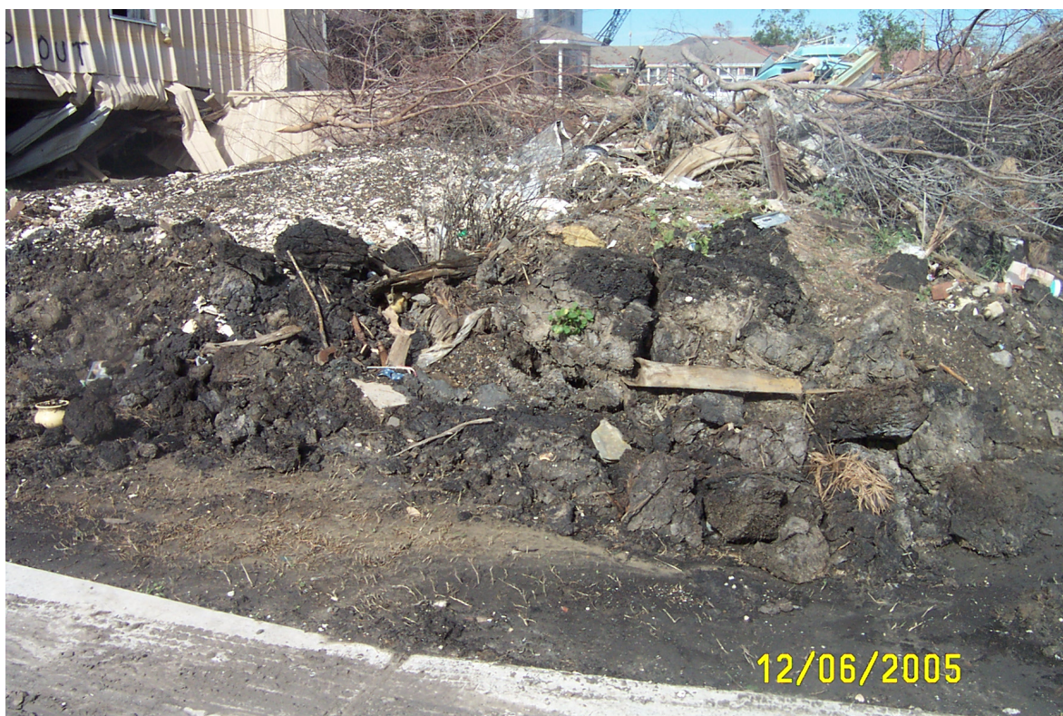
Figure 39. Blocks of Peat along Belaire Drive near the 17 th St. Canal levee breach
