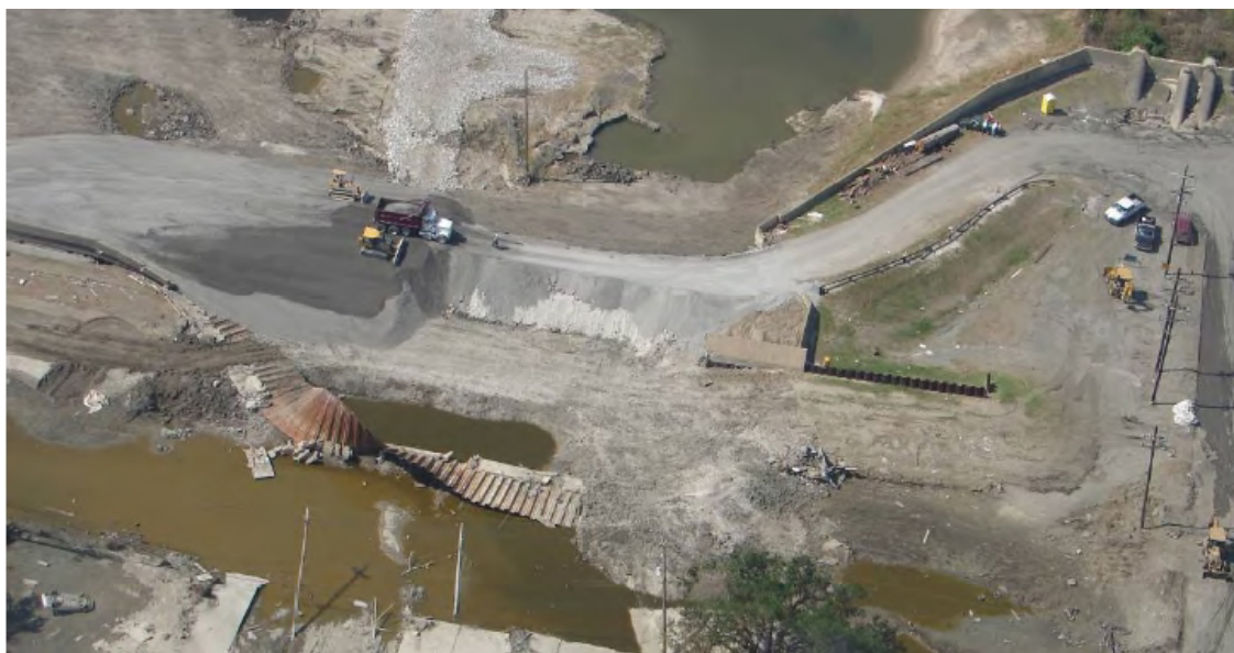
Figure 15. Aerial view of the north breach on Industrial Canal. Photo by L. Harder - Independent Levee Investigation Team Draft Final Report (2006).
