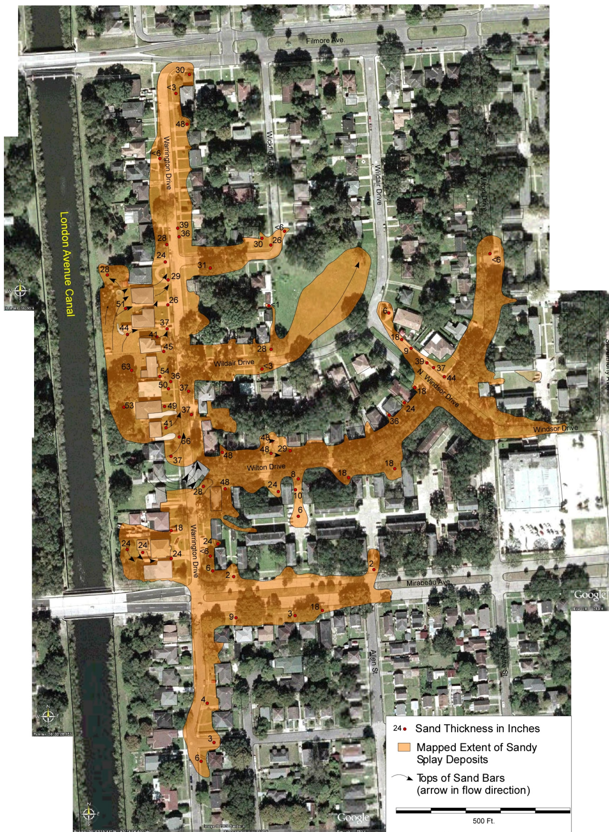
Figure 26. Preliminary map of sand deposits (by S. A. Nelson) from the Mirabeau Ave. Breach on the London Ave. Canal. Underlying image is a composite from Google Earth.
