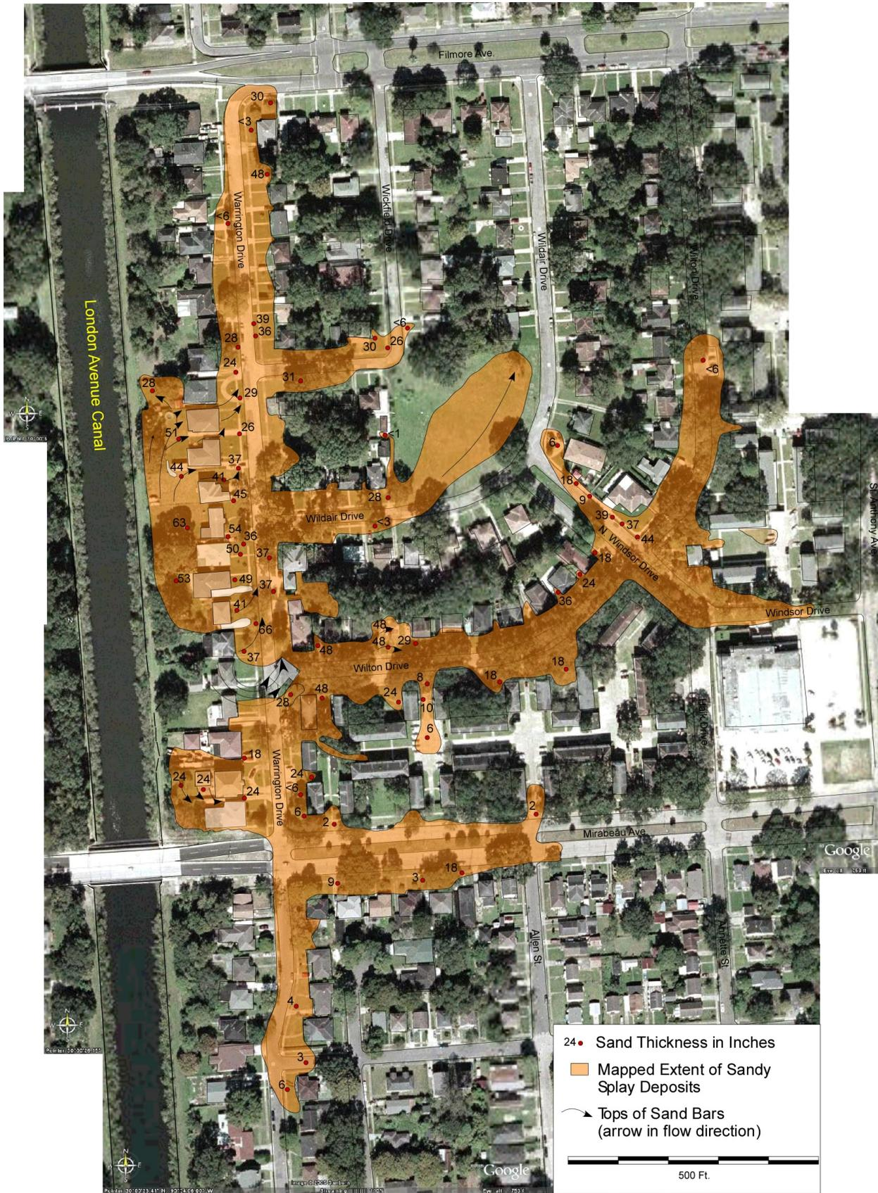
**Figure 20.** Preliminary map of sand deposits (by S. A. Nelson) from the Mirabeau Ave. Breach on the London Ave. Canal. Underlying image is a composite from Google Earth.
