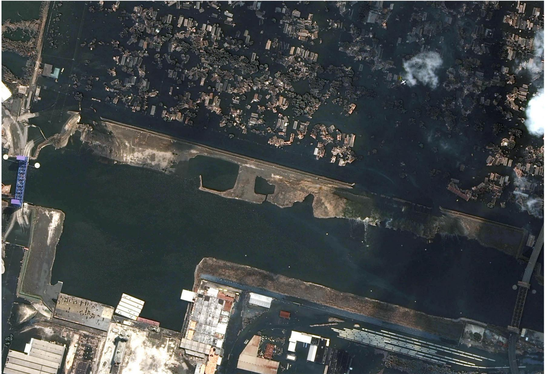
**Figure 10.** Air photograph of the area where the Industrial Canal Levee was breached to flood the Lower Ninth Ward. Image acquired Sept. 3, 2005
