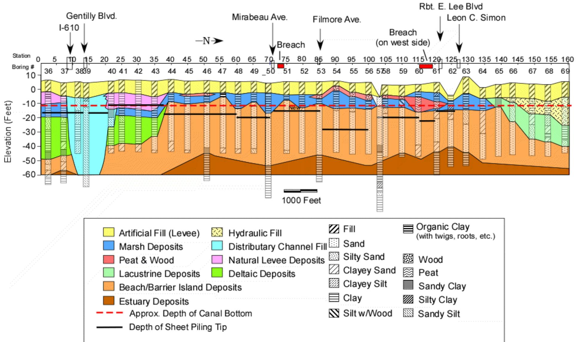
Figure 16. Geological cross-section along the east side of the London Avenue Canal constructed from data in U.S. Army Corps of Engineers (1989).
