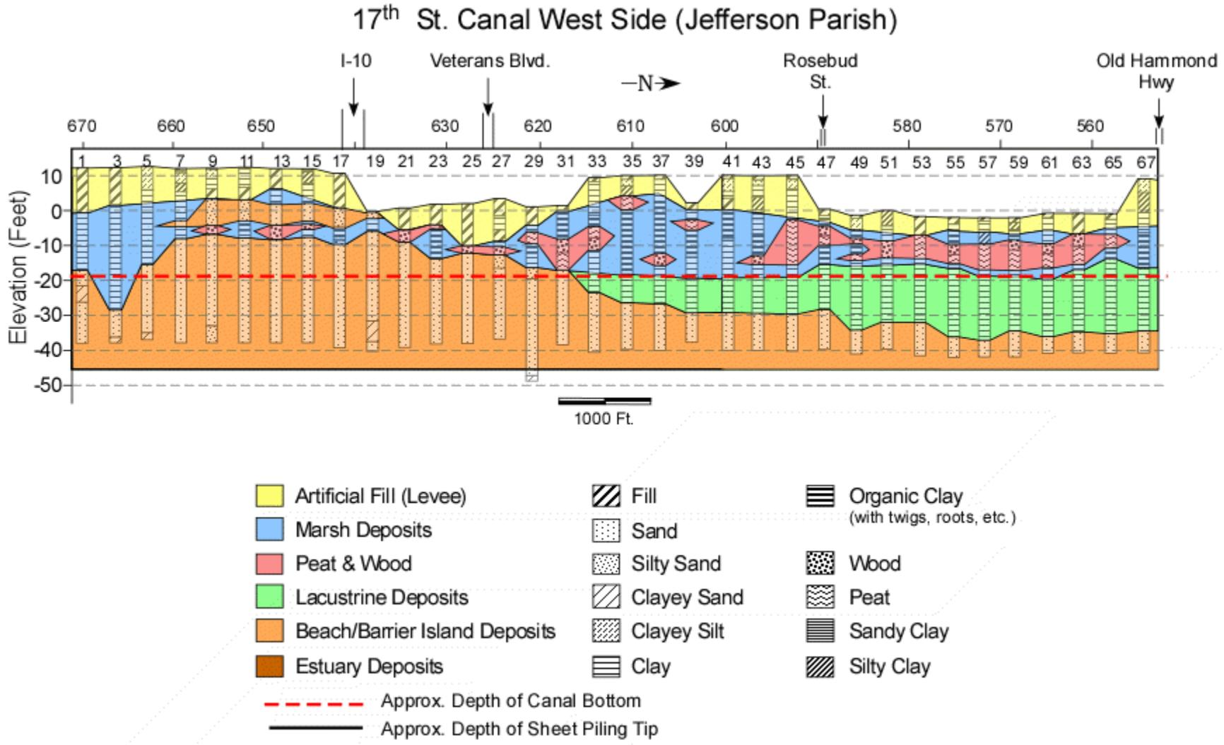
**Figure 32** Geologic cross section of the west bank of the 17<sup>th</sup> St. Canal constructed from data provided to the U.S. Army Corps of Engineers (1990).
