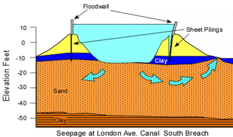
**Figure 18.** Geological cross section across the London Ave. Canal based on borings 16 and 51 (Figs. 15 and 22), shown at time of estimated high water during Katrina's storm surge. The sands form a permeable layer through which groundwater originating in the canal can penetrate and move below the sheet pilings and up to the surface, eventually undermining the levee and leading to its collapse.
