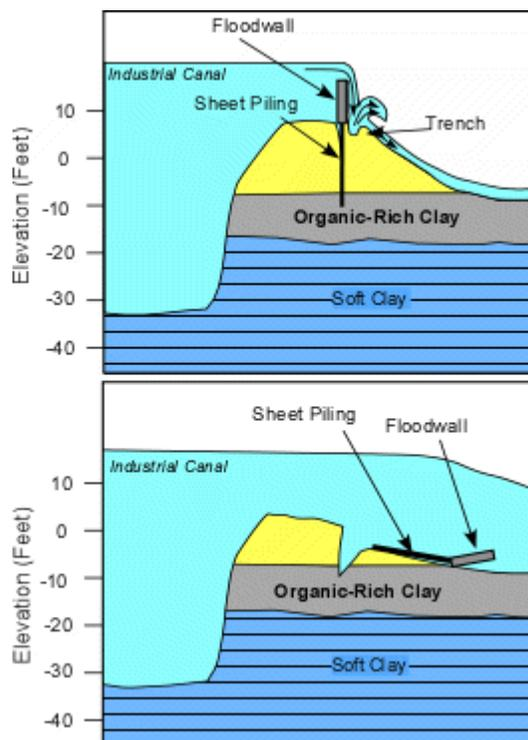
**Figure 13.** Possible failure mechanism at the Industrial Canal Levee breach in near the Lower 9<sup>th</sup> Ward.
