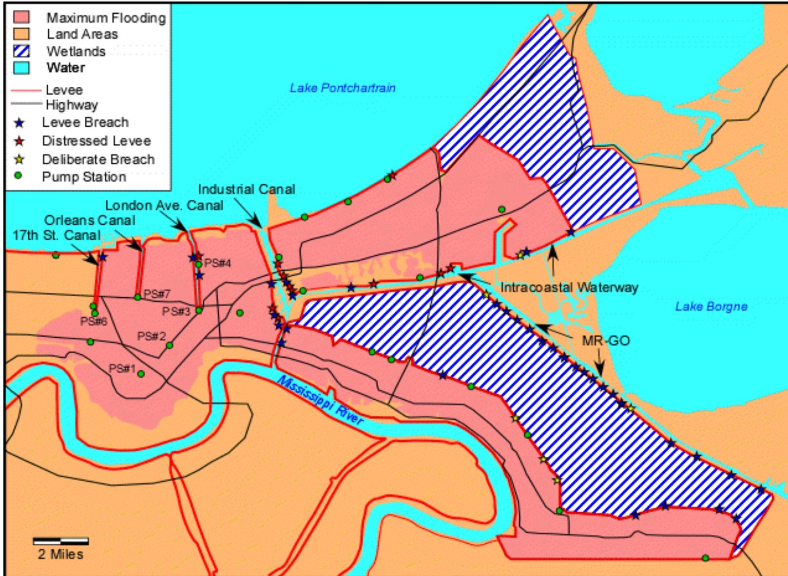
**Figure 7.** Map of maximum extent of floodwaters during Katrina modified and locations of breached levees after U.S. Army Corps of engineers-
