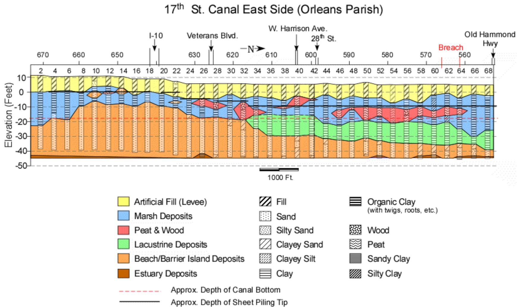
**Figure 28.** Geological cross-section along the eastern side of the 17<sup>th</sup> St. Canal (based on data in the U.S. Army Corps of Engineers design documents (1990). Notable in the cross-section is the peat layer that occurs in the area of the breach.
