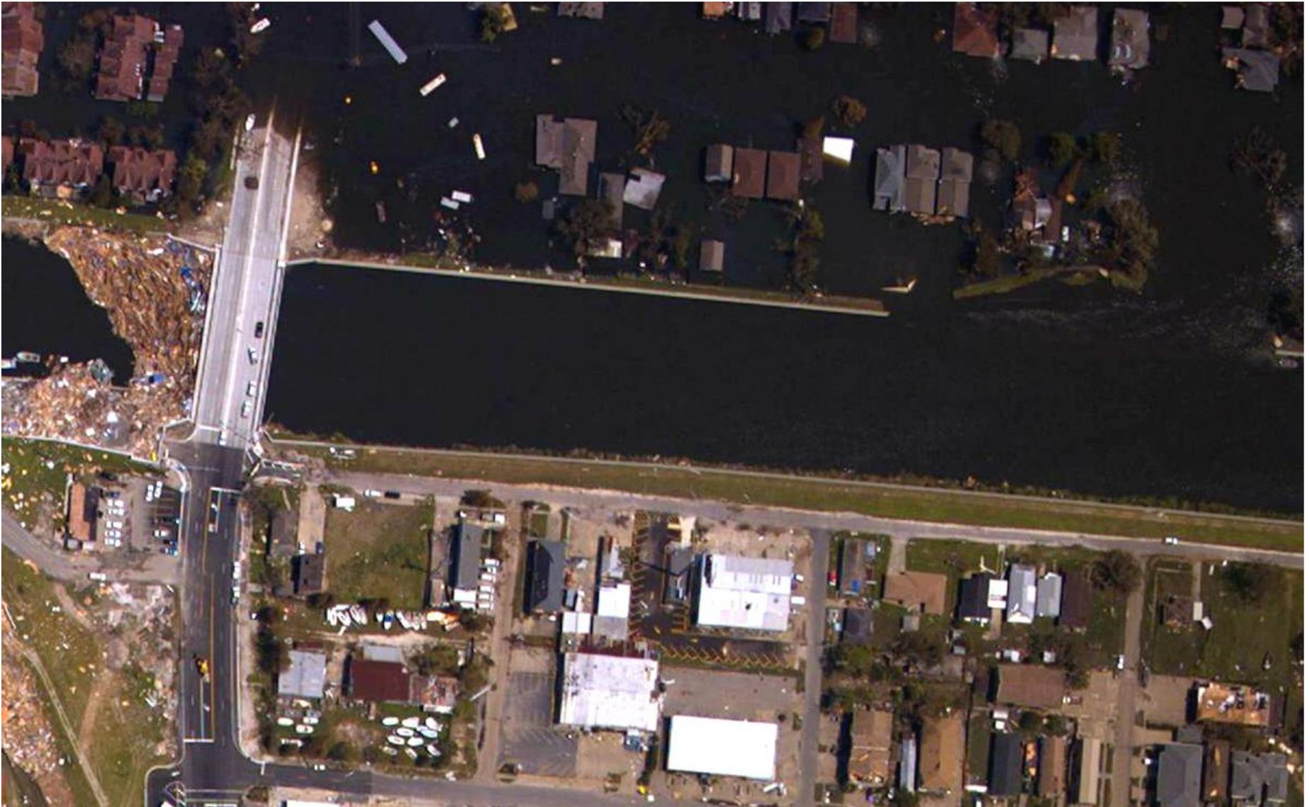
**Figure 27.** Air photograph of the area where the 17th Street Canal Levee was breached near Belaire Drive (stop 4). Image acquired Aug. 31, 2005. Source: National Oceanic and Atmospheric Administration's National Geodetic Survey, Katrina Images - <http://ngs.woc.noaa.gov/katrina/>
