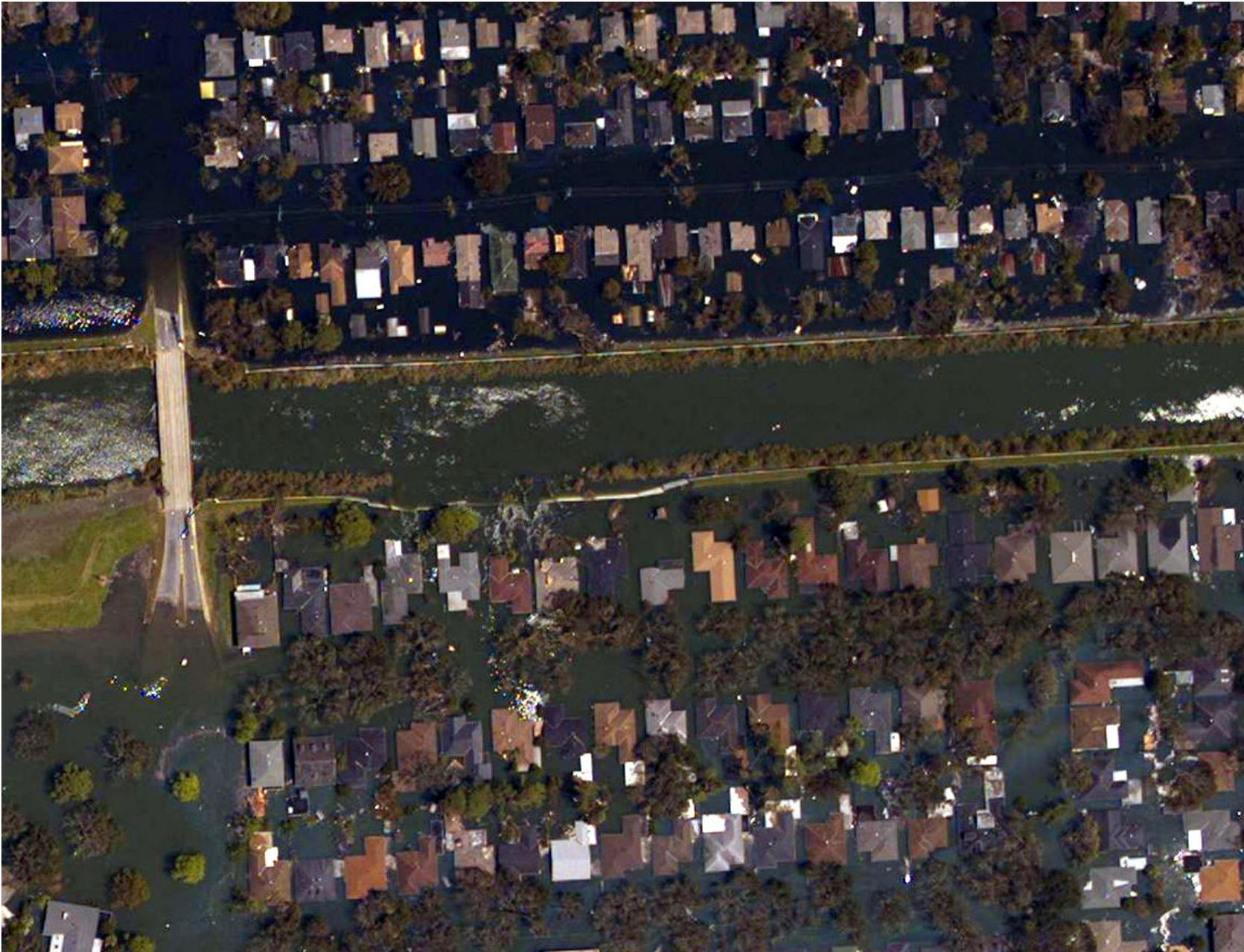
**Figure 22.** Air photograph of the area where the London Avenue Canal levee was breached near Robert E. Lee Ave. and Pratt Drive (Stop 2). Drive. Image acquired Aug. 31, 2005. Source: National Oceanic and Atmospheric Administration's National Geodetic Survey, Katrina Images - <http://ngs.woc.noaa.gov/katrina/>
