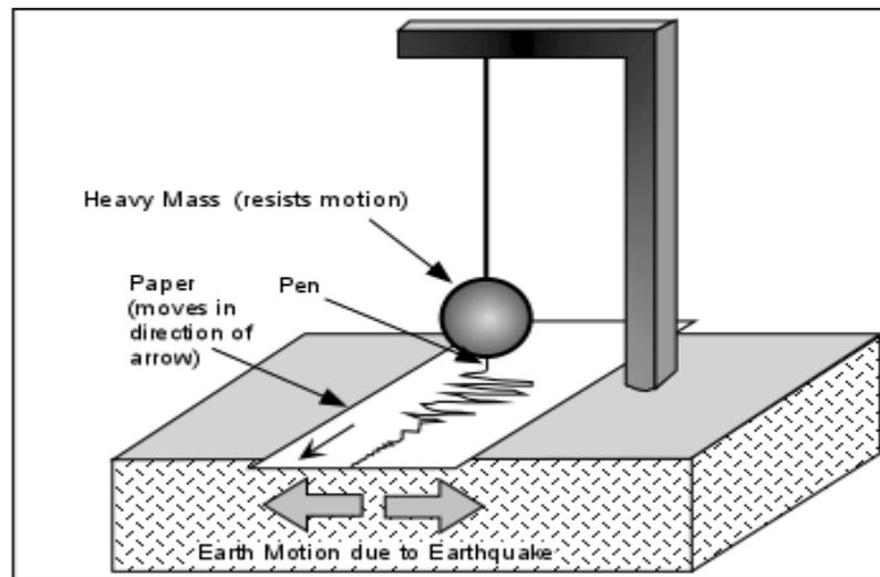
This is accomplished by isolating the recording device (like a pen) from the rest of the Earth using the principal of inertia. For example, if the pen is attached to a large mass suspended by a wire, the large mass moves less than the paper which is attached to the Earth, and on which the record of the vibrations is made. Modern instruments are digital and don't require the paper.
