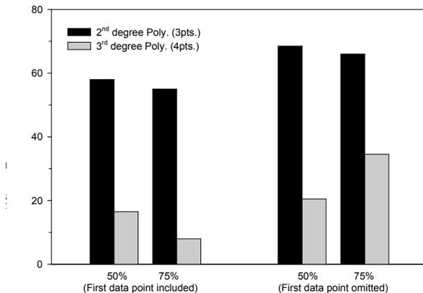
**Figure 3. Effect of velocity profile fitting function on shear stress measurement accuracy.**
