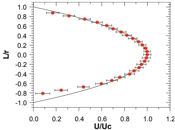
**Figure 2. Comparison of echo-PIV and analytic velocity profile (• : Echo-PIV, - : from analytic solution)**
