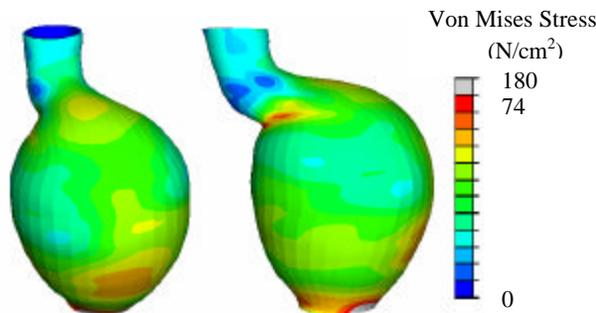
**Figure 2. Colored coded von Mises stress distribution, scaled to a maximum of 74 N/cm<sup>2</sup>**
