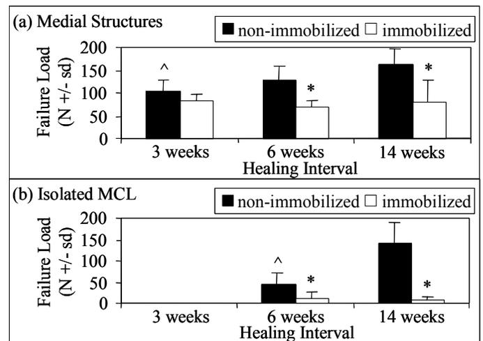
**Figure 1. Failure loads of (a) combined medial structures (medial capsule plus MCL) and (b) isolated MCL following isolated MCL injury**
