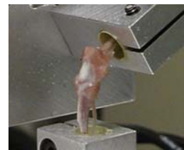
Figure 1. Dissected knee in custom testing fixtures. The joint capsule and the fibula are left intact. Proximal femur and distal tibia and fibula are potted in bone cement.
