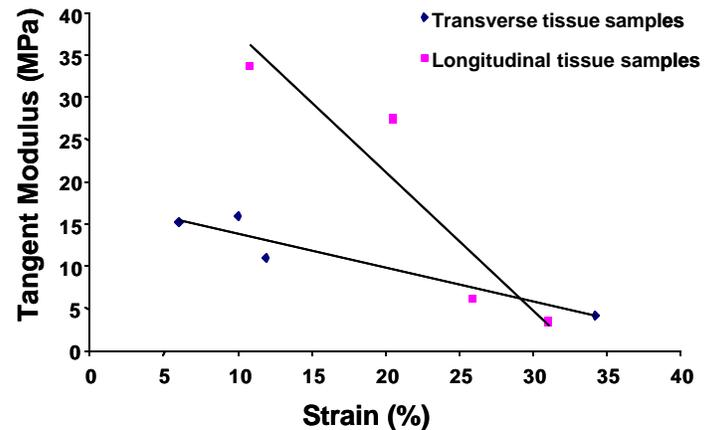
Figure 2. Linear correlations between the strain at failure and the tangent modulus of the transverse and longitudinal tissue samples.
