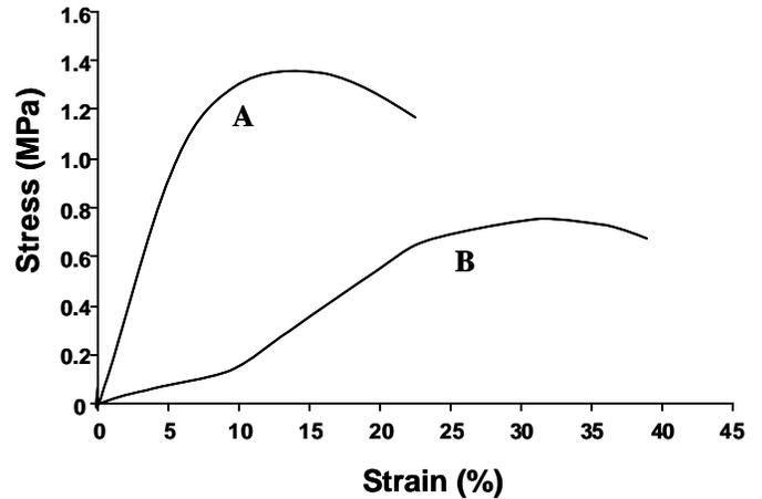
Figure 1. Typical stress-strain curves for the posterior capsule in the: A) transverse and B) longitudinal directions.
