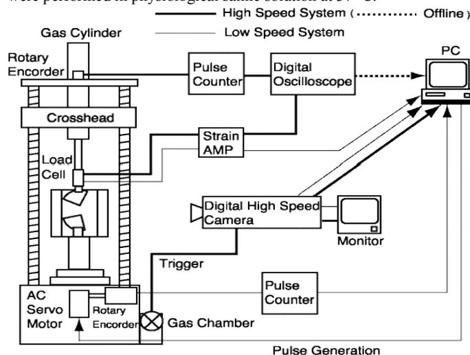
Figure 1. Schematic diagram of tensile test system
