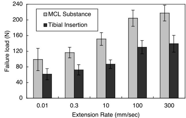
**Figure 3. Strain-rate dependency of failure load of tibial insertion and mid substance of MCL**
