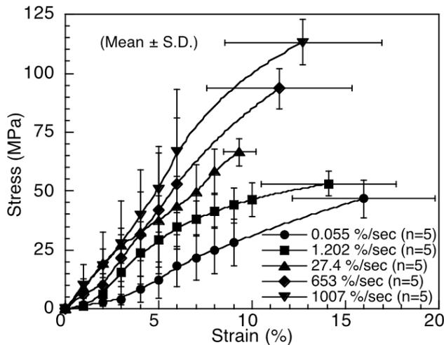
**Figure 2. Stress-strain curve of MCL substance**
