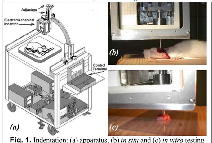
Fig. 1. Indentation: (a) apparatus, (b) *in situ* and (c) *in vitro* testing
