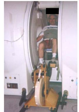
Figure 1. 59 y.o. pedaling a custom MR-compatible exercise cycle in a GE 0.5T open magnet.
