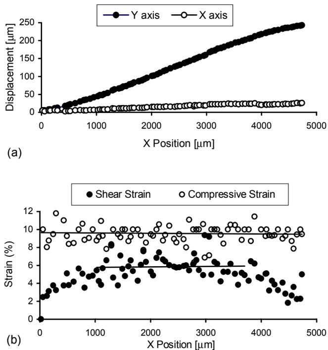
**Fig. 2 Displacement of cells parallel (Y) and perpendicular (X) to the axis of shear (a) and the resulting local shear and compressive strains (b) across the specimen length. Linear models have been fitted to the strain data. For shear strain, only points within the central region of the specimen (>1mm from each end) were included.**
