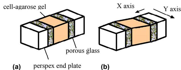
**Fig. 1 Schematic diagram showing the cell-agarose specimen gelled between porous glass in the unstrained state (a) and with an applied shear strain in the Y axis (b).**
