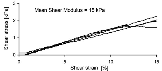
**Fig. 3 Shear stress - strain response for 4% cell-agarose constructs.**
