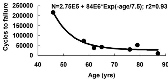
**Figure 1: Age-related change in the fatigue life of human cortical bone subjected to bending fatigue. Each point in the figure represents an average of two specimens obtained from the anterior and posterior cortex of tibial diaphysis.**
