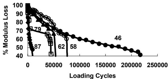
**Figure 2: Percent modulus loss versus loading cycles for human cortical bone specimens from 5<sup>th</sup> to 9<sup>th</sup> decades.**
