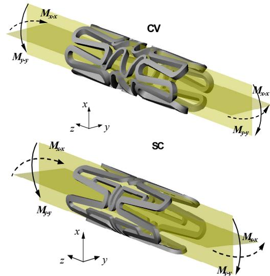
**Figure 1. Geometry of the two stent units studied and planes of application of the bending moment.**
