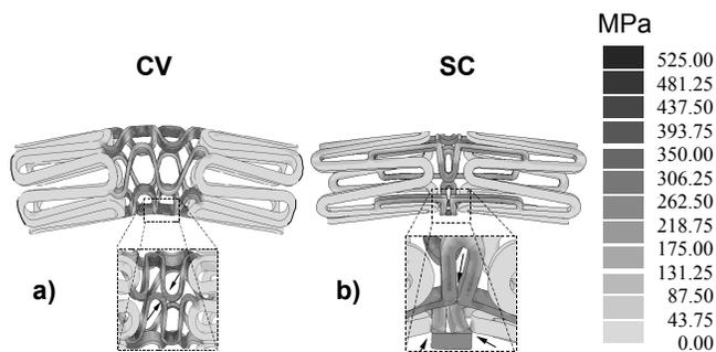
**Figure 3. Von Mises stresses ( $\chi = 0.06 \text{ rad}\cdot\text{mm}^{-1}$ ) for the CV (a) and SC (b) models in the unexpanded configuration during the bending around the  $x$  axis. Arrows in the enlargements reverse view indicate the areas of contact.**
