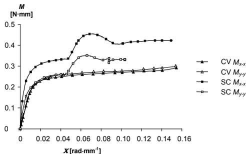
**Figure 2. Moment-curvature index curves for the unexpanded configurations of CV and SC models.**
