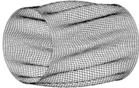
Figure 1. Buckling pattern of a thin-walled tube under torsion.
