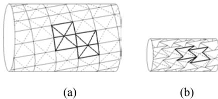
Figure 2. One of the folding patterns with helical folds for tubular stents. (a) It is fully expanded and (b) completely folded.
