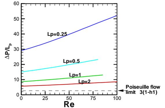
Figure 4. Driving Pressure drop divided by the plug length.
