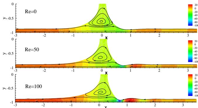
Figure 3. Streamlines and Pressure Fields.
