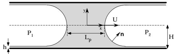
Figure 1. Liquid Plug Model
