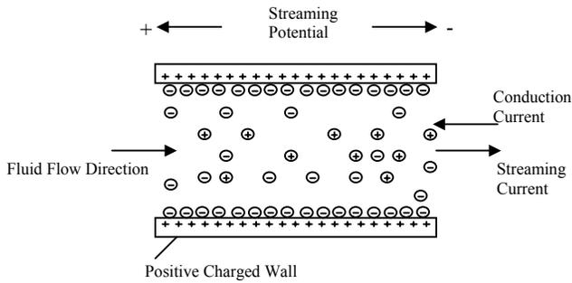
**Figure 2. Streaming Potential and Current in Microfluidic Channel**
