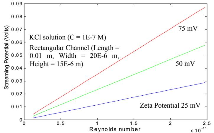
**Figure 3. Calculated Streaming Potential**
