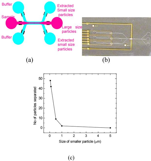
Figure 2 (a) Extraction of particle in MHD network bioassay by diffusion. (b) Image of MHD micropump. (c) Simulation Results with H- filter series
