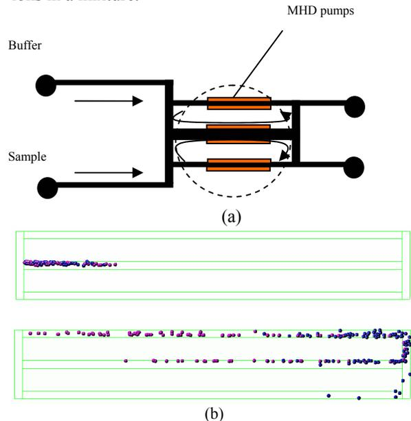
Figure 3 (a) Schematic of cyclic H filter. (b) Simulated results in the initial configuration and after one cycle circled parts in a.
