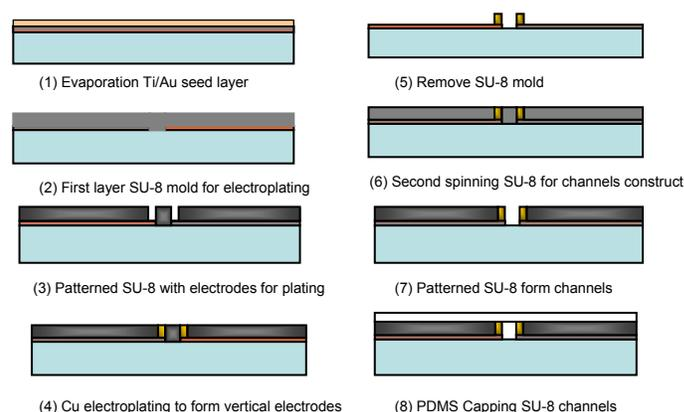
Figure 1 Fabrication processes of MHD micropumps
