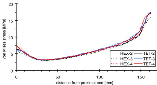
Figure 2. Initial stress state in lateral cement mantle
