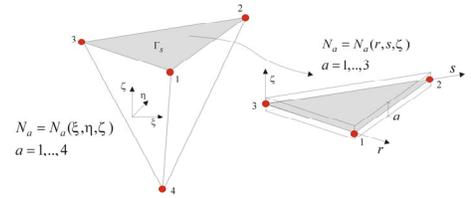
**Figure 3. Diagram of a typical boundary element showing the set of shape functions used to characterize the fluids domain (left) and the solids domain (right)**
