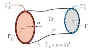
Figure 1. Boundary decomposition for the Coupled Momentum approach.
