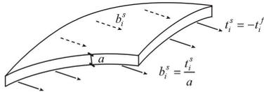
**Figure 2. Relationship between the surface traction due to the fluid motion  $t_i^f$  and the solids body force  $b_i^s$ .**
