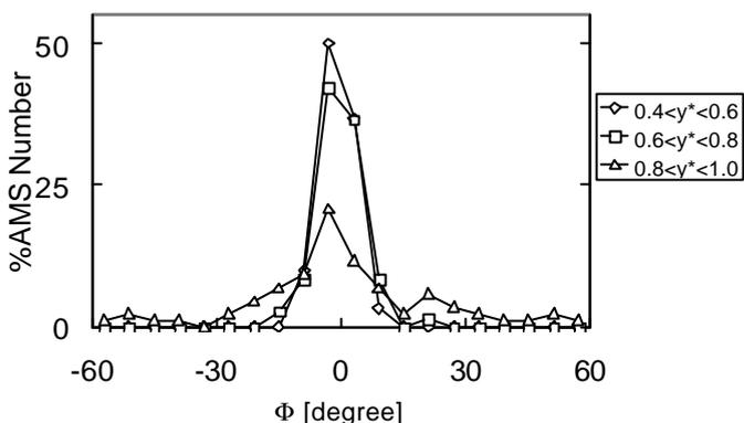
Figure 4. Histogram of drift angle of particle motion in the flow. We should note the profile tends to be flat near the wall.
