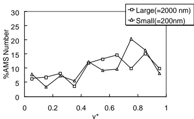
Figure 3. Effect of particle size on the concentration profile with the shear rate of 190 sec<sup>-1</sup>
