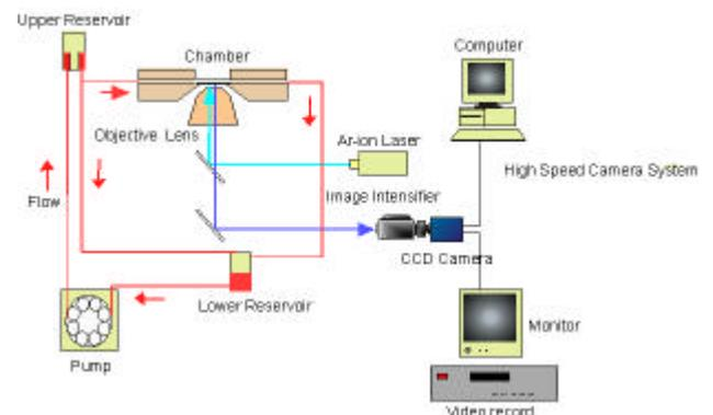
Figure 1. Experimental system to visualize the microscopic motion of artificial platelets flowing in the model arteriole
