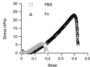
**Figure 2: Stress-strain relationship for biogels incubated in the absence or presence of FN (40 nM)**
