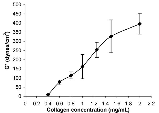
**Figure 2. Complex shear modulus of varying concentrations of collagen gels determined using rheology. Error bars are standard deviation from the mean where n≥4.**
