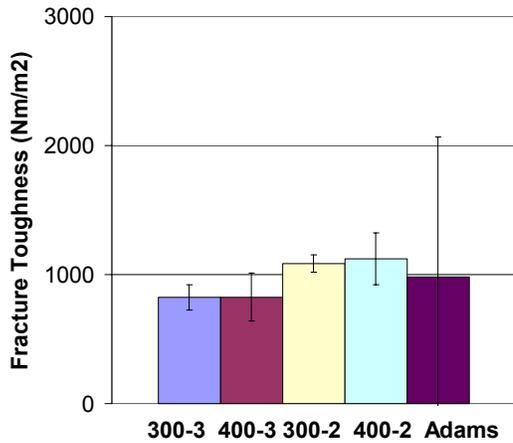
**Figure 2: Predicted fracture toughness for 300 and 400 mN maximum load, and as measured by Adams et al. [3].**
