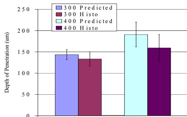
Figure 1: Penetration depth predicted by the method and measured by histology.
