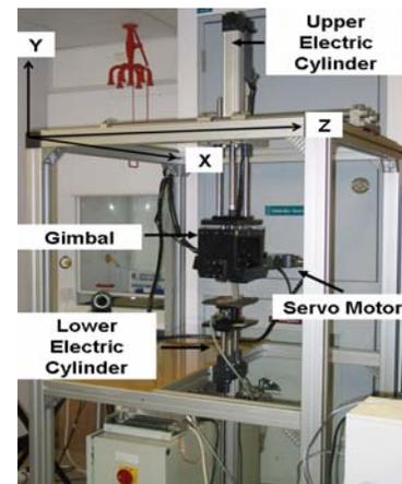
Figure 1: Overview of the loading system
