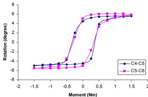
Figure 2: Primary motion of the C4-C6 spine specimens.
