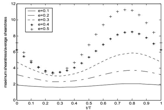
Fig. 5 Maximum wall shear stress for various constriction coefficient  $\epsilon$  and at  $f=120/\text{min}$
