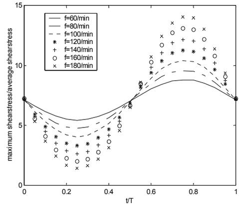
Fig.3 Maximum wall shear stress for various constriction moving frequency  $f$  and at  $\epsilon = 0.5$
