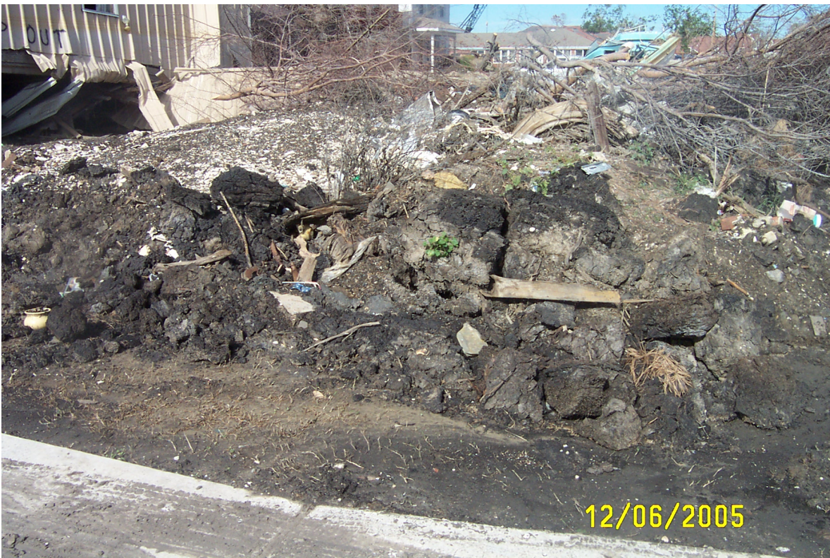
Figure 44. Blocks of Peat along Belaire Drive near the 17 th St. Canal levee breach
