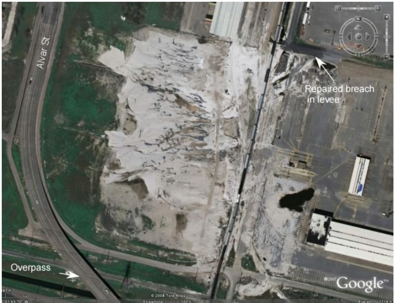
Figure 24. Google Image (acquired around May, 2006) of area near overpass to Alvar St. (point A in Figure 1) showing location of breached levee and deposits of shells (white material in center of image) that resulted from the breach. Industrial Canal is off the image to the right (east).
