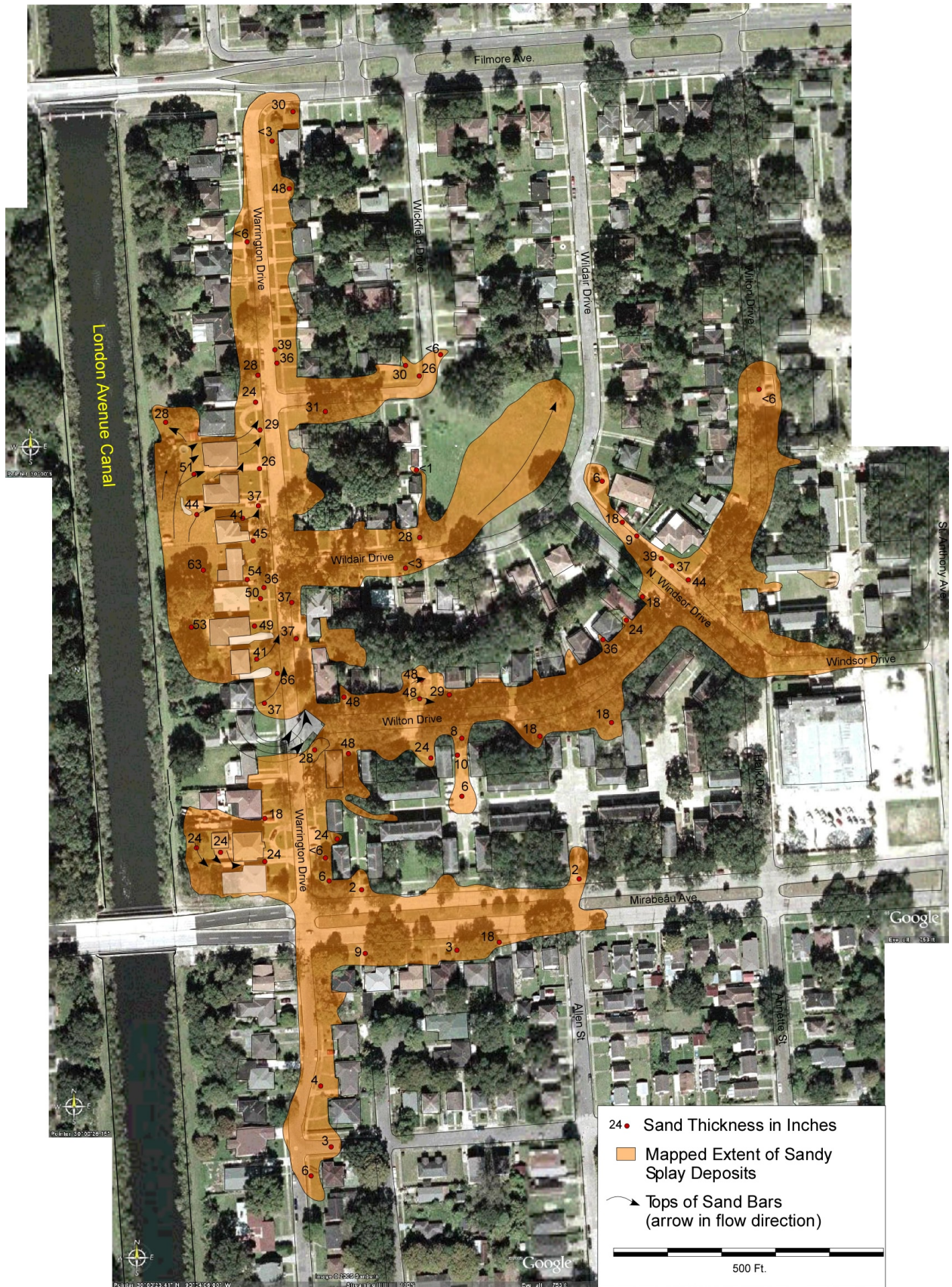
Figure 23. Preliminary map of sand deposits (by S. A. Nelson) from the Mirabeau Ave. Breach on the London Ave. Canal. Underlying image is a composite from Google Earth.
