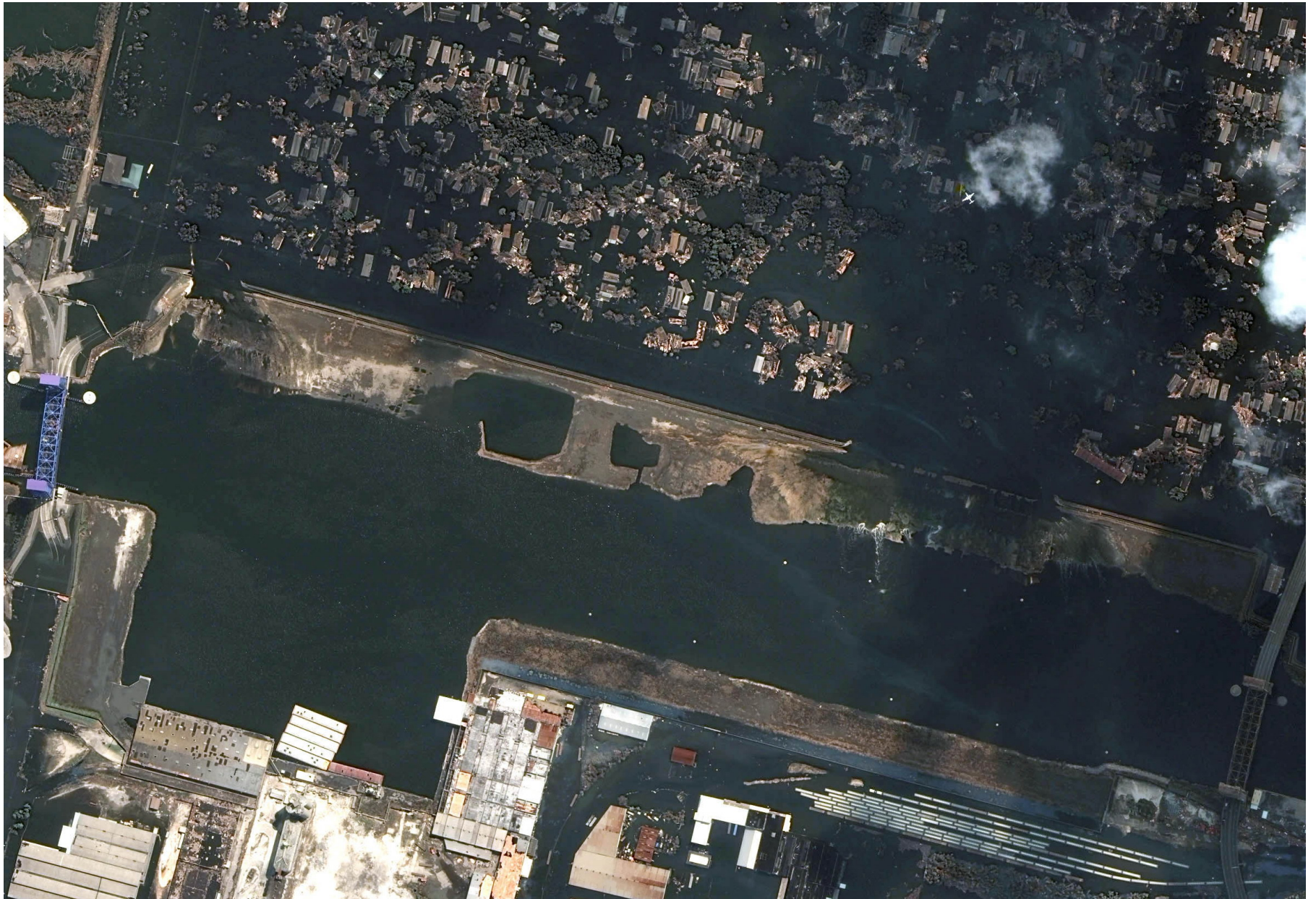
Figure 10. Air photograph of the area where the Industrial Canal Levee was breached to flood the Lower Ninth Ward. Image acquired Sept. 3, 2005 Source: National Oceanic and Atmospheric Administration's National Geodetic Survey, Katrina Images - http://ngs.woc.noaa.gov/katrina/
