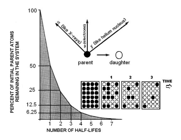
Radioactive isotopes decay to stable daughther isotopes while emmiting radiation or particles or both. The rate of decay is expressed as the half-life, the time it takes half of the parent isotope to decay to the daughter isotope. The rate is exponential, as can be seen on the decay curve above. The curve at first drops very rapidly, then much slowly.
