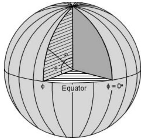
As an example, the  $\rho$  and  $\phi$  angles for the (111) crystal face in a crystal model is shown here. Note again that the  $\rho$  angle is measured in the vertical plane containing the **c** axis and the pole to the face, and the  $\phi$  angle is measured in the horizontal plane, clockwise from the **b** axis.
