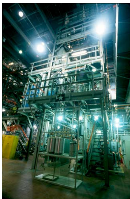
Figure 8 Large 1.5 bbl/d riser pilot plant used in the development of the PCC Process
