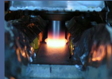
High Temperature Friction Stir Weld
