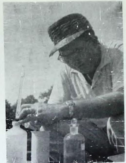
River Doctor Jack W. Sadler is pictured making a test to determine the amount of oxygen in the water during one of the regular trips down the Ouachita River.
